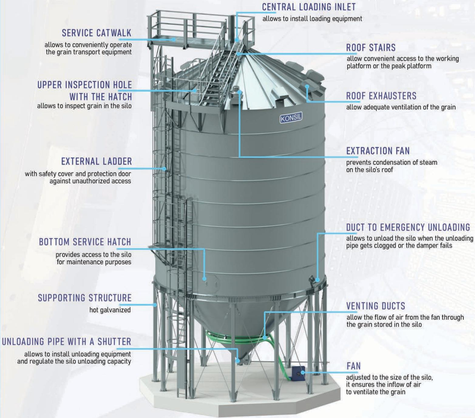
The equipment is different in different silo models.
